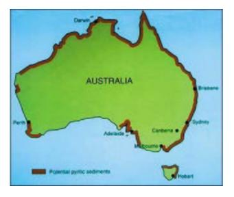
Figure 1. Coastal acid sulphate soils in Australia. (original source, National Strategy for the Management of Coastal Acid Sulphate Soils, January 2000) [deh, 2004].
